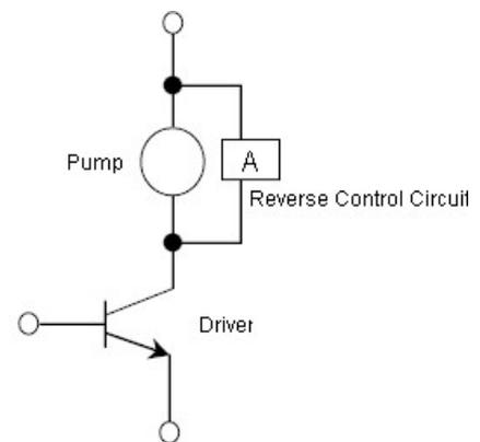
Fig.4: Reverse Voltage Protection Circuit
