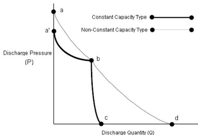
Fig.1 P-Q Characteristic Curve
