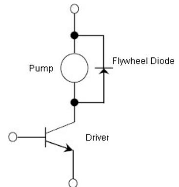
Fig.3: Reverse Voltage Protection Circuit
